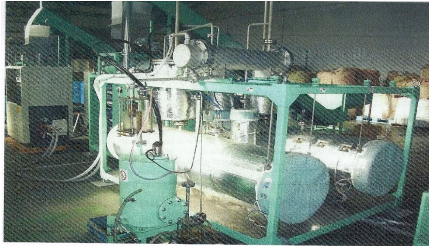
A photograph of the Nagata Shigyou Fukaya Clean Center NGV 2000 2.5 tons of plastic per day machine The green frame around the reactor is 71" wide, 158" long and 55" high
